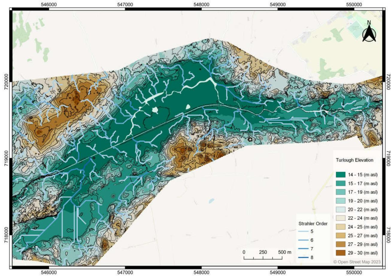
Figure 3-3: Map of key drainage network, overlain on 50 cm contours generated from the 2m lidar DEM
